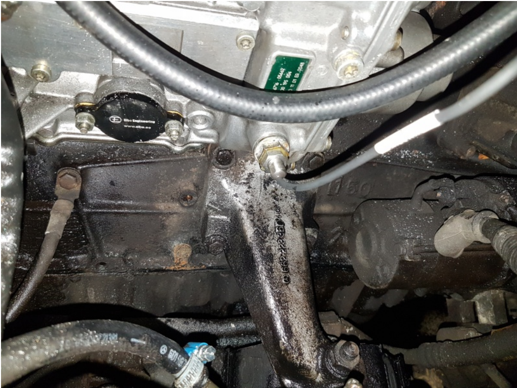
Figure 4.4: Honeywell LCZ260 sensor installed in injection pump
