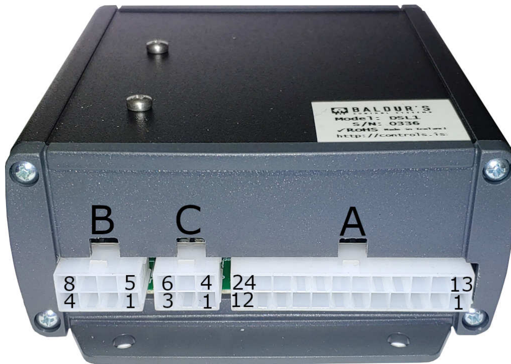
Figure 2.3: Pin numbers of connectors on back of controller.
