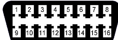
Figure 3.1: OBD2 female connector as seen from the end the scan tool plugs in to.
