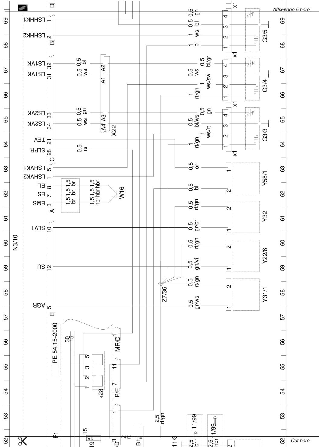
Wiring diagram - ME-SFI fuel injection and ignition system / pe07.61-p-2000-99ag
