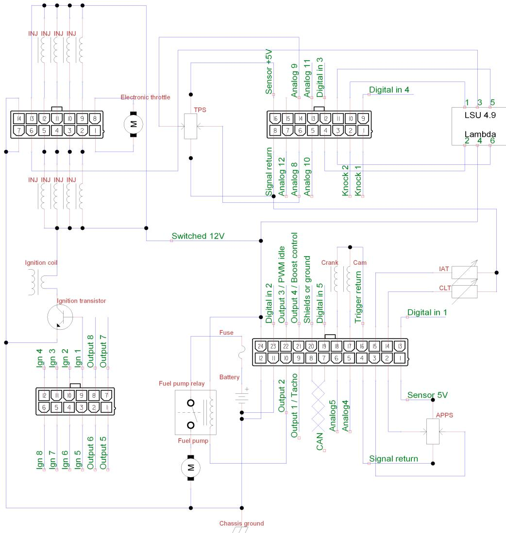
Figure 2.3: Typical wiring with electronic throttle.
