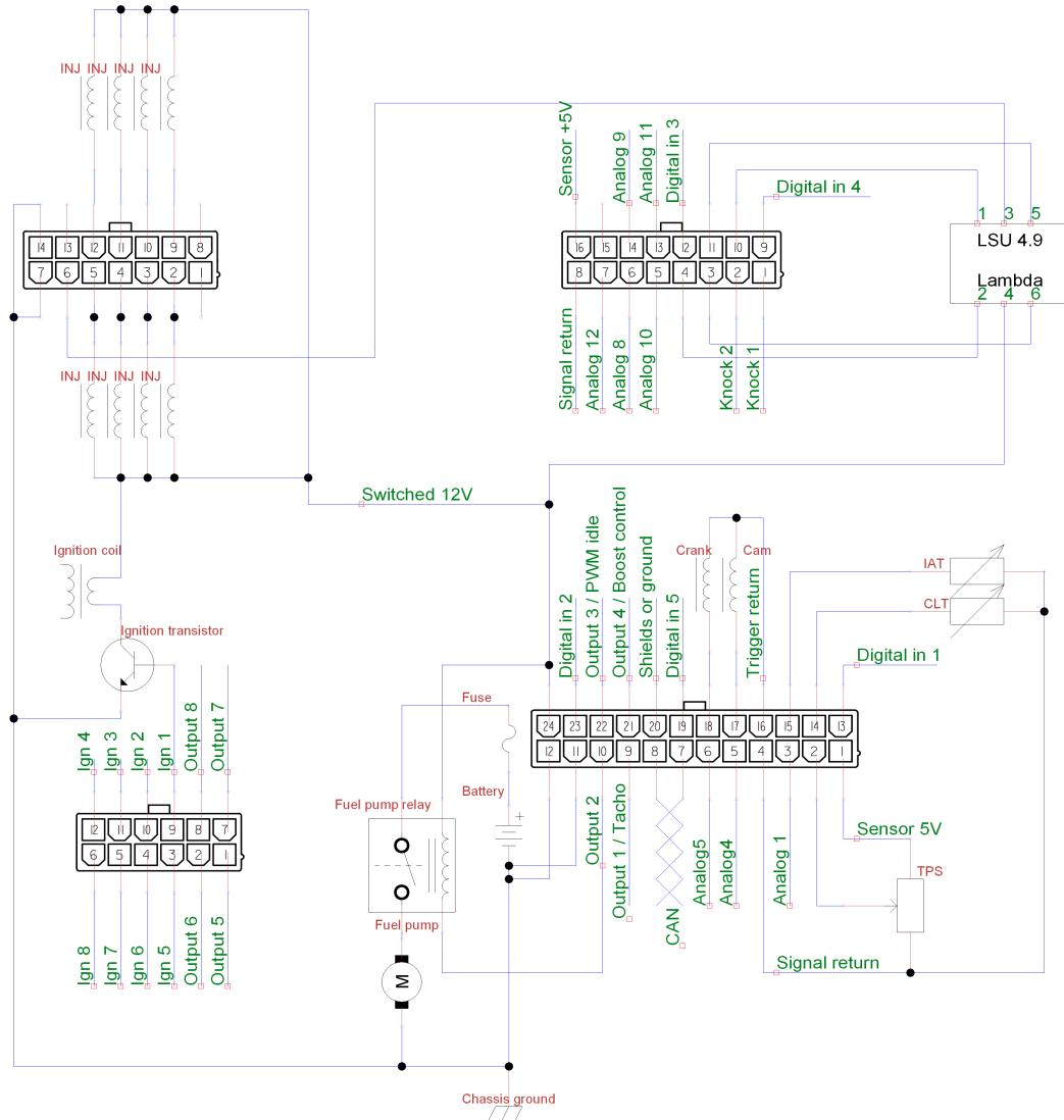
Figure 2.2: Typical basic wiring
