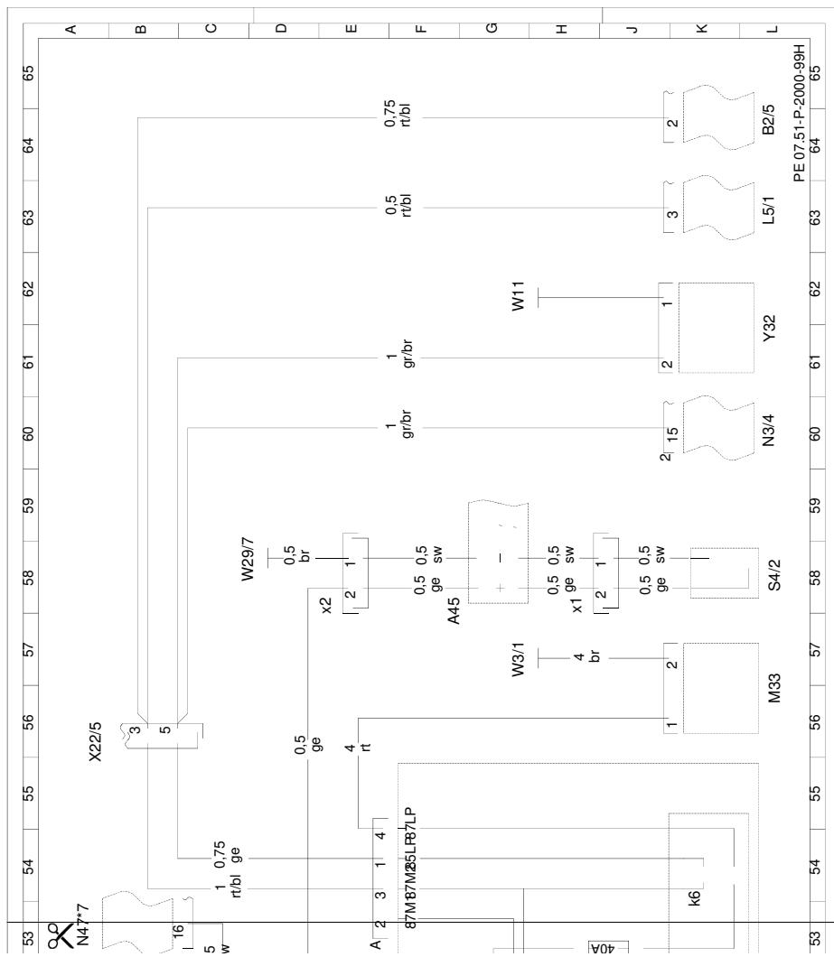
Wiring diagram HFM-SFI sequential multiport fuel injection/ ignition system / pe07 51-p-2000-99h
