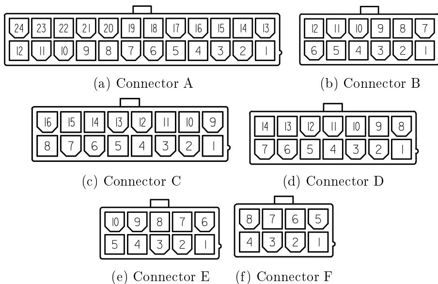
Figure 2.1: Pin numbering of the different connectors on the back of the controller. Note that the connectors are not oriented as shown but the locking tabs face inwards. Connector E only present on units with second lambda sensor option, located on front panel above USB port. Connector F also located on the front, present on units with serial number 2200 and above.
