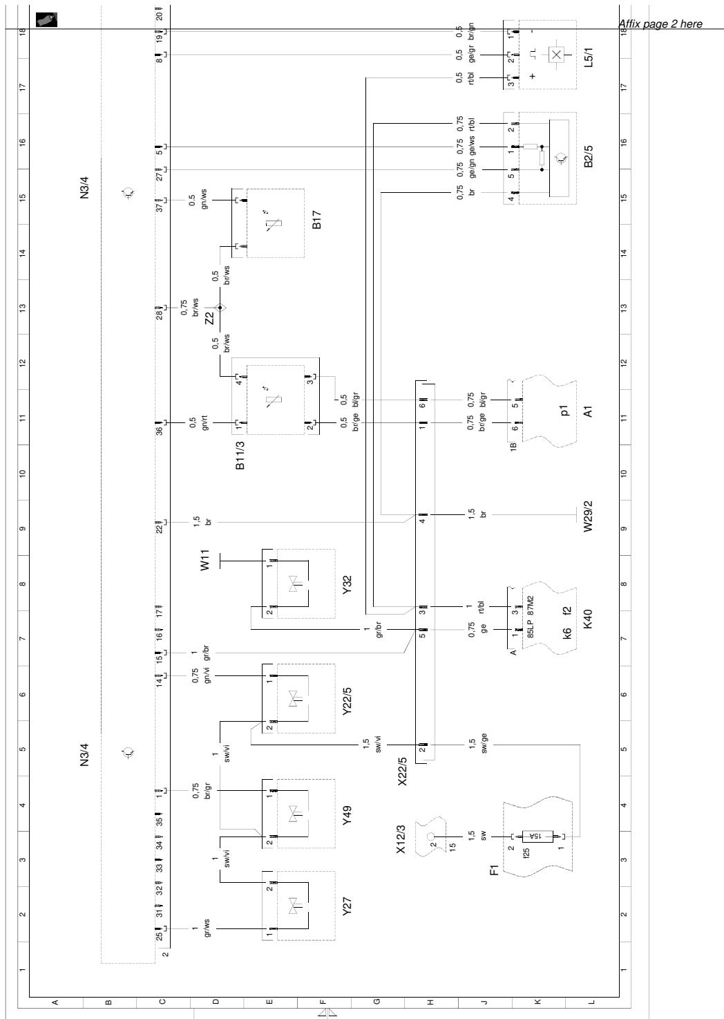
Wiring diagram HFM-SFI sequential multipoint fuel injection/ ignition system / pe07.51-p-2000-99i
