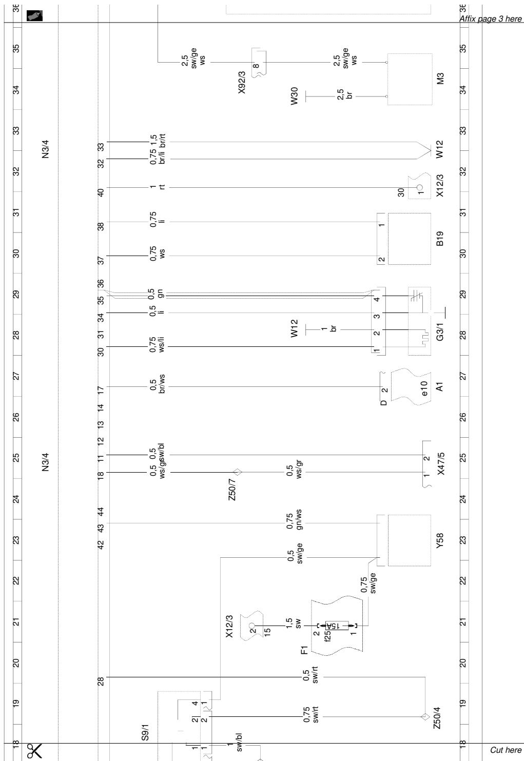
Wiring diagram HFM-SFI sequential multiport fuel injection/ ignition system / pe07 51-p-2000-99h
